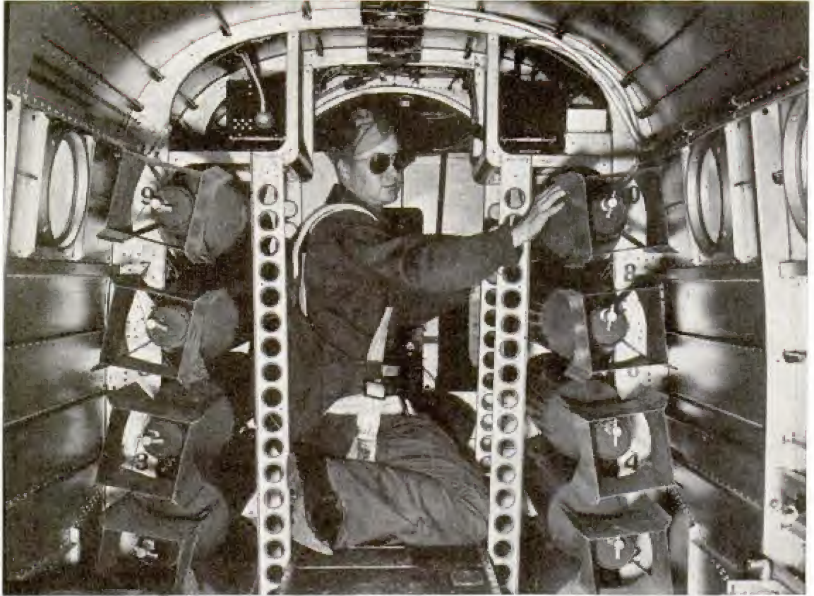
The bombardier checks arming wires on 100-pound practice bombs in racks of a training plane, above. Left, putting the precious bombsight into the "greenhouse" while an armed guard stands by
